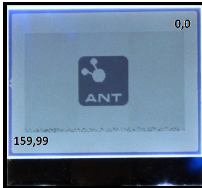
Figure 4.1.1: Picture of working LCD screen with pixel address shown
